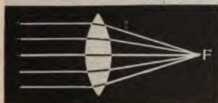
FIG. 151.—The Action of a Convex Lens on Parallel Rays.
